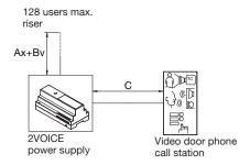
C = distance between the power supply and the call station
