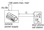
C = distance between the power supply and the call station
