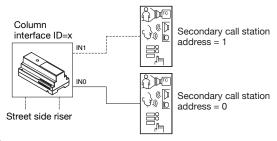
In one-column systems with one main and one secondary call station directly connected to the column interface, devices must be connected and configured as follows:
