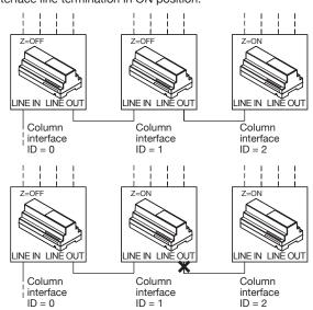
In the example shown in the figure, the interface with ID=2 is separated from the rest of the system, so the interface with ID=1 becomes the last one and must have the line termination active.
