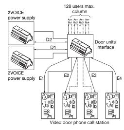
Ex = distance between the door units interface and the call station Dx = distance between the door units interface and the power supply
