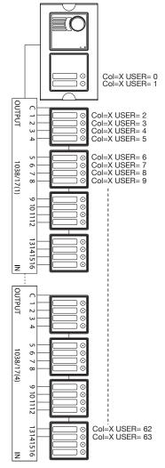
If door units are configured as secondary, but each station must call a different group of users, it is possible to follow the procedure indicated for each call station in respective sections.
