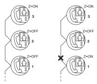
In the figure, the apartment stations 2 and 3 are separated from the rest of the system, so the apartment station 1 becomes the last one and must have the line termination active.
