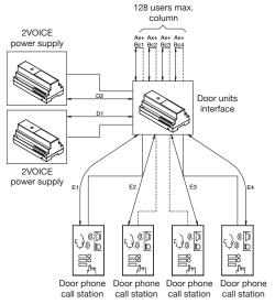
Ex = distance between the door units interface and the call stationDx = distance between the door units interface and the power supply
