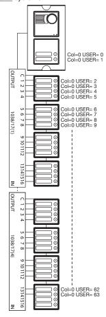
If the door unit is configured as main and in the system there are <u>more than one column</u>, buttons and column users must be associated, following the procedure indicated for each call station in respective sections.
