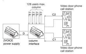
Cx = distance between the column interface and the call station
