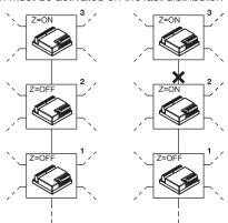
In the example, the distributor 3 is separated from the rest of the system, so the distributor 2 becomes the last one and must have the line termination active.
