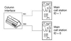
• In case of <u>secondary call station</u>, the ID must be the same as the column ID configured on the column interface.
