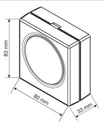
The electronic ringer Ref. 9854/40 can be used as additional ringer: the call coming from the door unit activates both the apartment station ringer and the additional ringer Ref. 9854/40.
