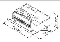
The device Ref. 788/22 allows to implement the call repeater function.
